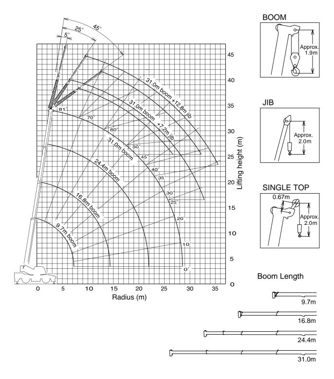
**NOTE:** The above lifting height and boom angle are based on a straight (unladen) boom, and allowance should be made for boom deflection obtained under laden conditions. The above working range is shown on condition with outriggers fully (6.3m) extended.
