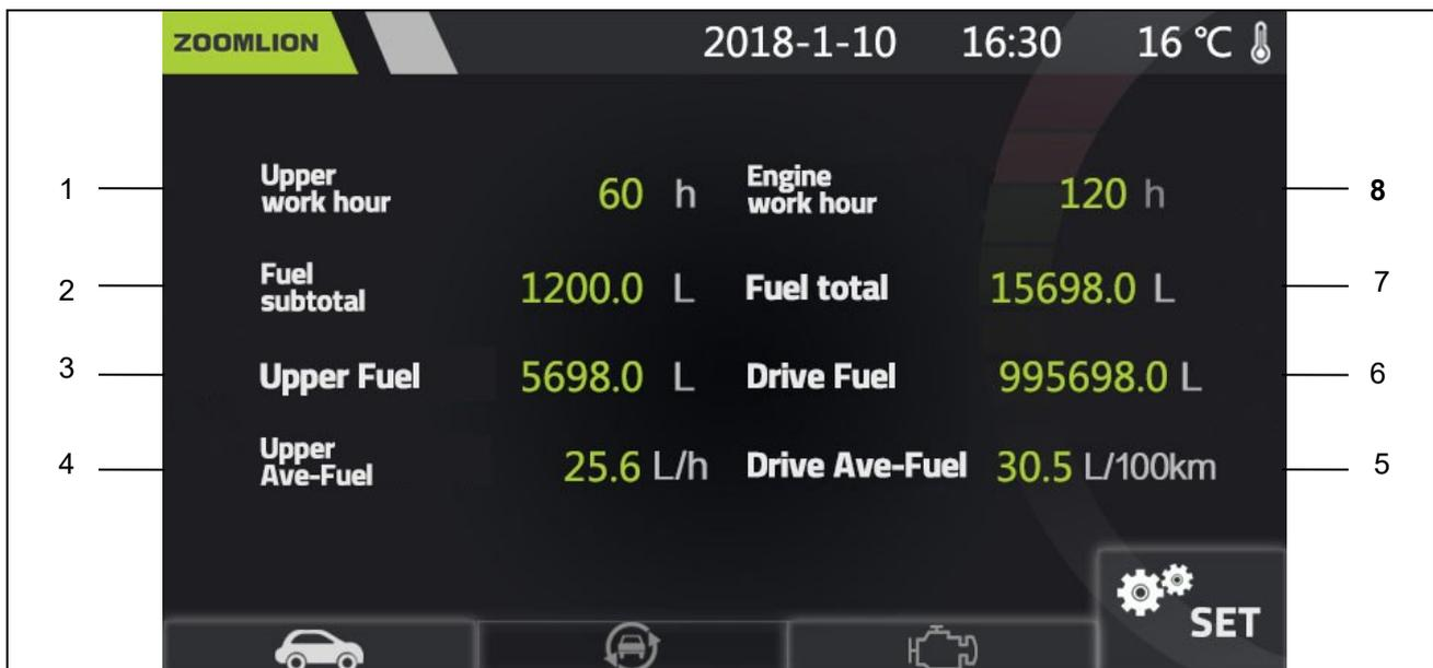
Figure 3-10 Secondary instrument interface
