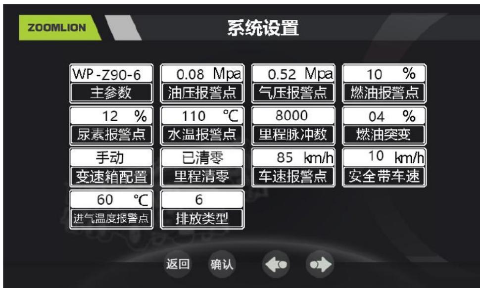
Figure 3-15 System parameter setting interface
