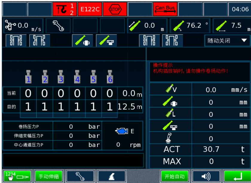
Figure 4-32 Telescopic boom section edit interface
