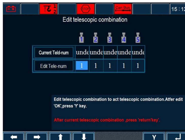
Figure 4-31 Telescopic boom section edit interface
