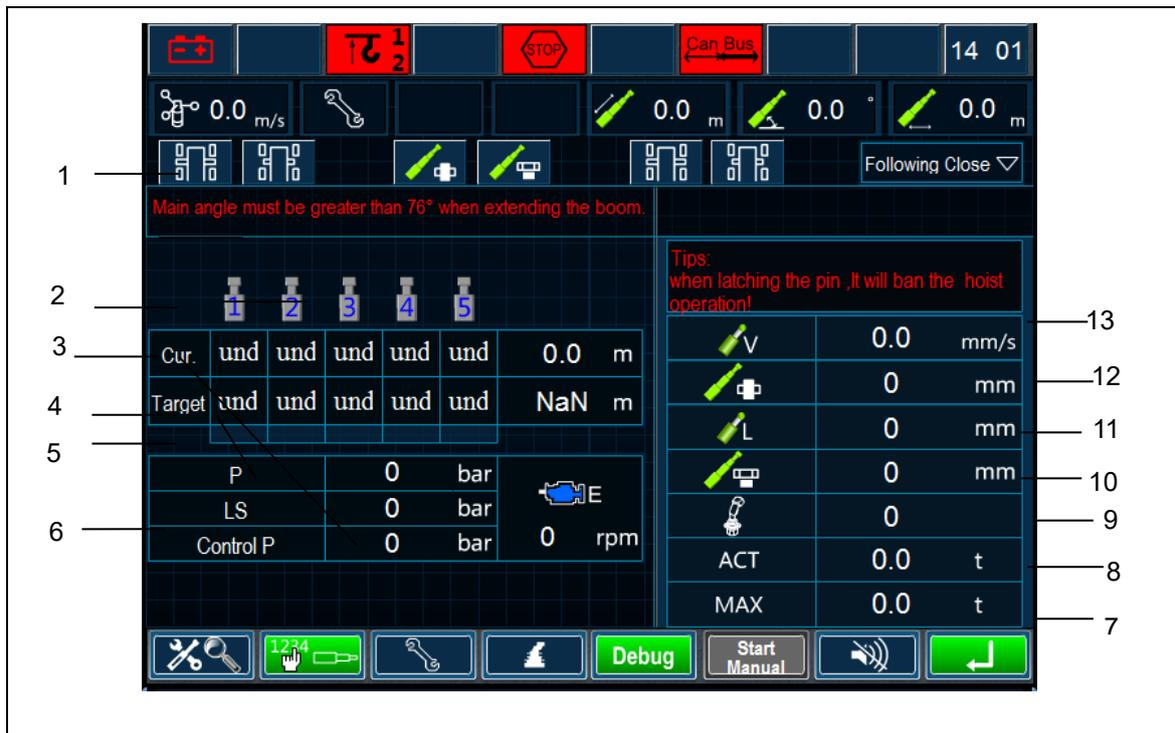
Figure 4-41 Boom status during manual telescoping
